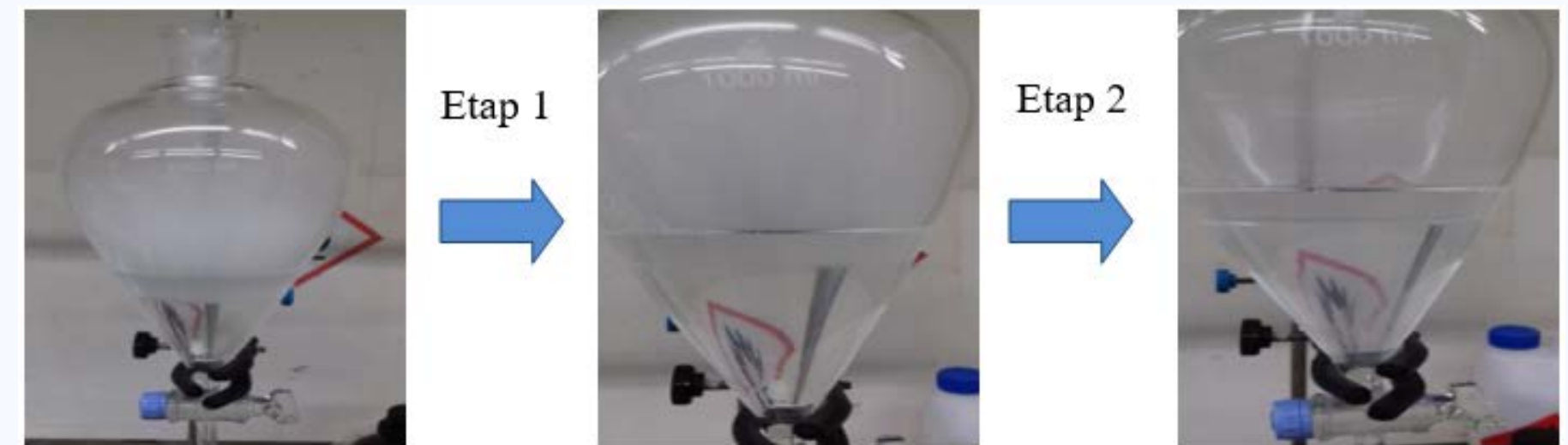
separation of the aqueous phase from the ether phase
