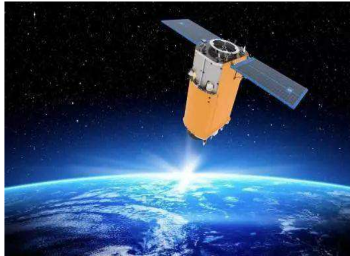
Jilin-1 Satellite Attitude pointing stability: 5 \times 10^{-4} / \text{s}
