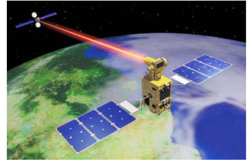
Laser Communication Satellite Attitude pointing error: 1 \mu rad
