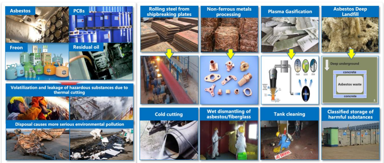
Figure 1. The novel approach and technologies of ship and offshore platforms recycling
