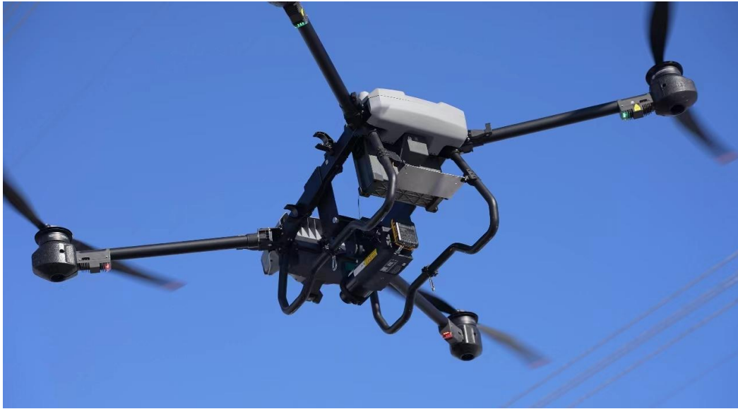
Fig 1: Heavy-lift UAV equipped with X-ray transmitter
