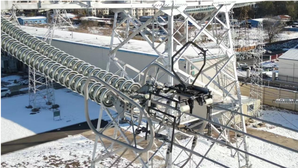
Fig 2: The movable imaging plate moves to the tension clamp inspection position
