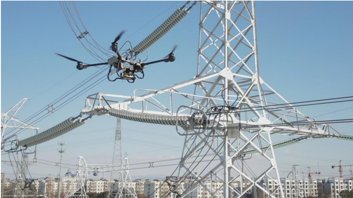
Fig 2: The movable imaging plate moves to the tension clamp inspection position
