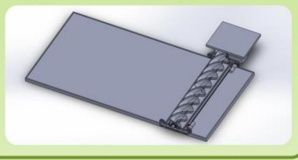
According to research, ready-made washing robots that work dry can clean up to 80% of the surface of the panels and remove dust from them. Cleaning the panels by this robot can increase the amount of force produced in increase the length of time by an average of 3.5%. This robot has a lower manufacturing cost than other robots, and the amount of energy consumed is less, and it also has no pollution.
