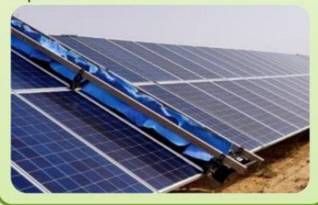
In general, this robot does the washing job completely and can make many improvements in the future in the direction of clean energy. To improve the performance of the panel washing robot, the material of the brush, its movement speed, and the number of brushes can be changed. Also, the design of a robot with the ability to change its dimensions to fit all types of panels is one of the suggestions to continue the process of this project.
