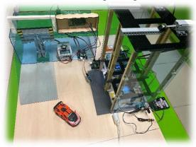
The water height inside and outside the parking lot is different, so we decided to set the water level sensor both inside and outside, to detect water level anytime.
